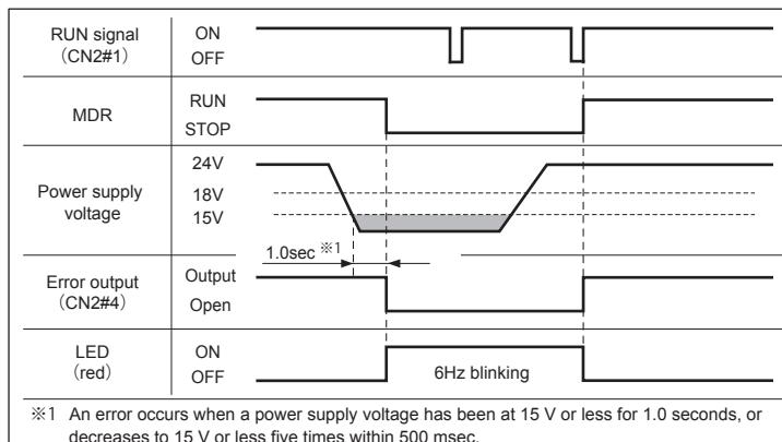
\*1 An error occurs when a power supply voltage has been at 15 V or less for 1.0 seconds, or decreases to 15 V or less five times within 500 msec.
