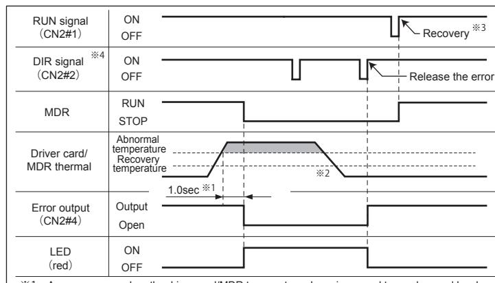
\*1 An error occurs when the driver card/MDR temperatures have increased to an abnormal level or higher for 1.0 seconds.
