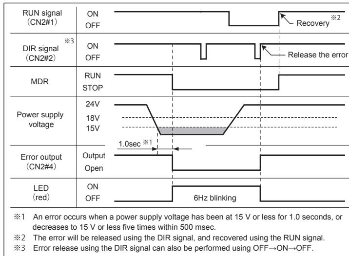
\*1 An error occurs when a power supply voltage has been at 15 V or less for 1.0 seconds, or decreases to 15 V or less five times within 500 msec.
