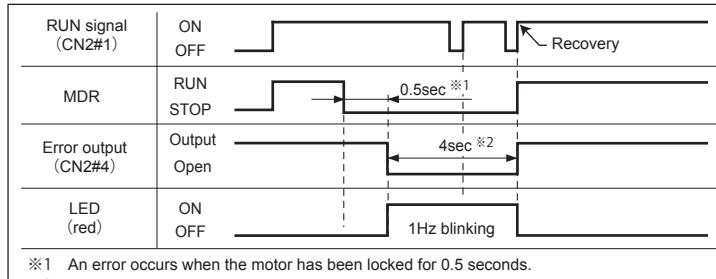
\*1 An error occurs when the motor has been locked for 0.5 seconds.
