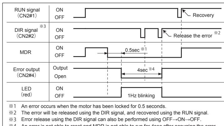
\*1 An error occurs when the motor has been locked for 0.5 seconds.
