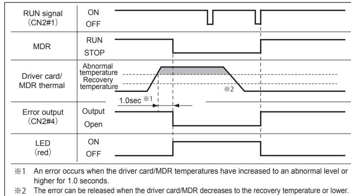
\*1 An error occurs when the driver card/MDR temperatures have increased to an abnormal level or higher for 1.0 seconds.
