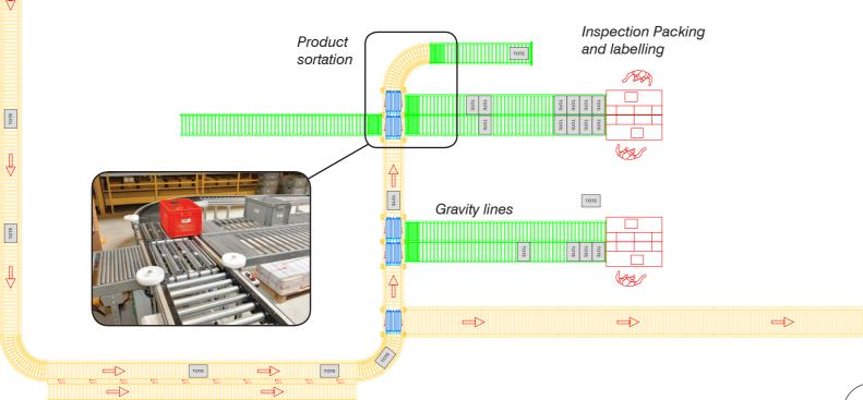
To acheive the required design aesthetic Amsort manufactured conveyor modules constructed from aluminium profiles which are scalable and very flexible to allow for remodelling and expansion of the system. The drive rollers and zone sensors are fully integrated within the profile along with the cabling. This means that the conveyor has very clean lines without mechanical protrusions usually associated with traditional drives or mechanical support legs.
