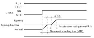
\*Reverse direction by DIP switch is prohibited while motor is running. Motor must be stopped first, and then reverse a direction by DIP switch.
